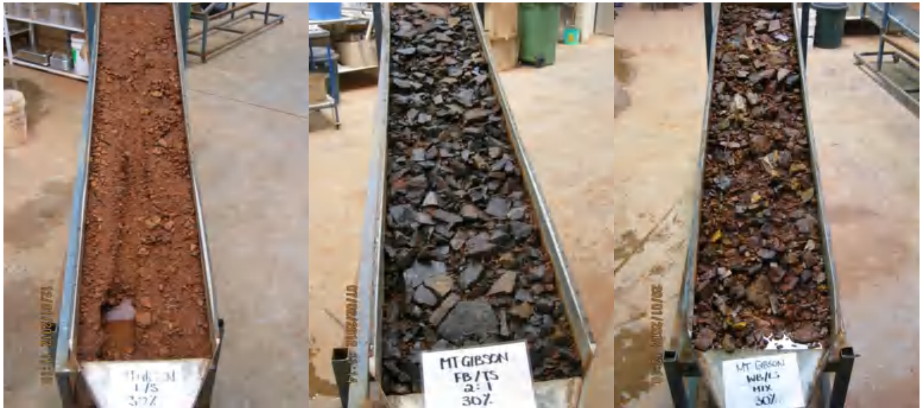
Figure 5: Surfaces after application of concentrated overland flows: Sandy soil (left), Fresh BIF/sand mix (middle), Weathered BIF/sand mixture (right).
